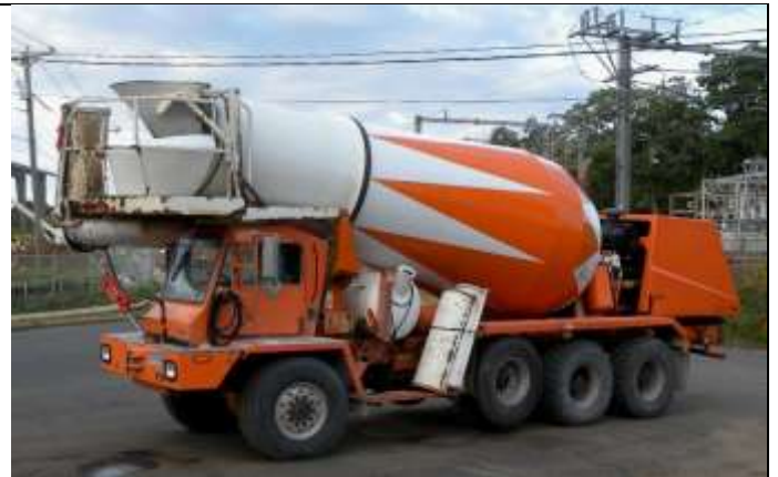
2. Concrete ready-mix truck including mixing drum, front discharge capability for improved access to placement, and water storage. (Schexnayder)
