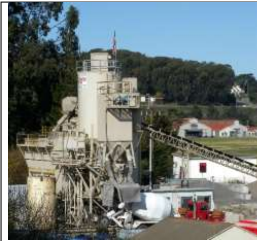
1. Concrete batch plant showing cement storage, aggregate hoppers, and discharge to ready-mix truck. (Schexnayder)
