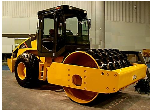
Figure 8. Padded drum vibratory compactor.
